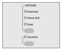
Select the desired "OPTIONS". Press the upper button until the indicator of the desired wash option lights.
